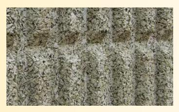
A porous lightweight aggregate-based cementitious material averaging 36-40 pounds per cubic foot
